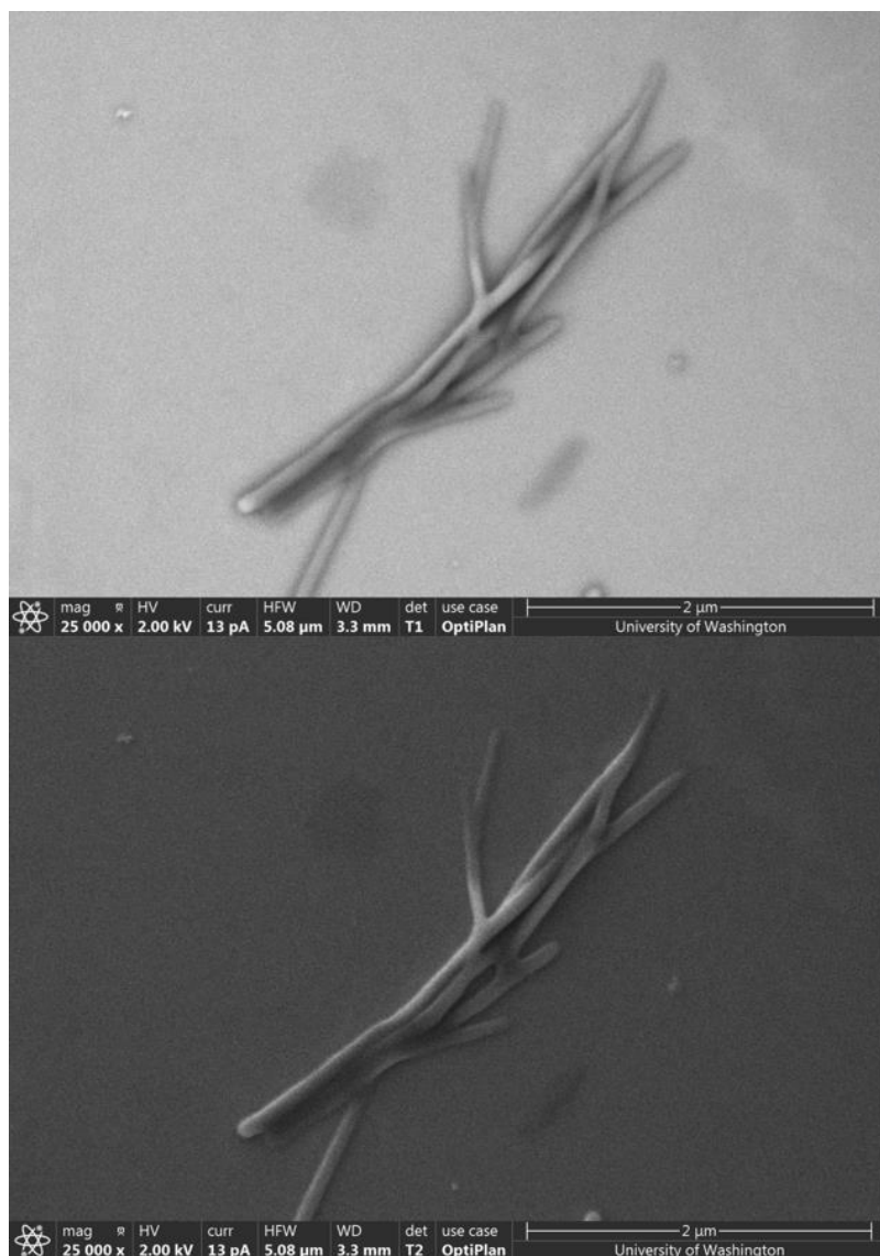
Figure 20. T1/T2 SEM images of materials purified from the hydrothermal synthesis of YLF with dopamine-HCl and ammonia added. Possibly hydrothermally synthesized PDA nanowires.
