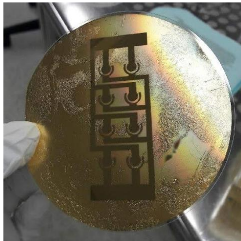
Figure 2.2 – Substrate held by a gloved researcher after the deposition of gold, highlighting the photopolymerized design visible at the center
