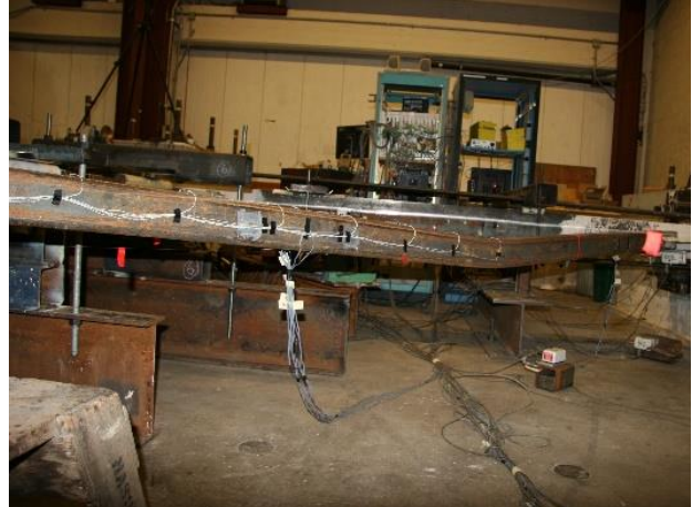
Figure 4.25 N Brace plastic deformation @ -2.8% drift
