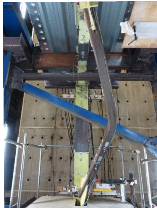
(b) 2SBr -2.25% roof drift
