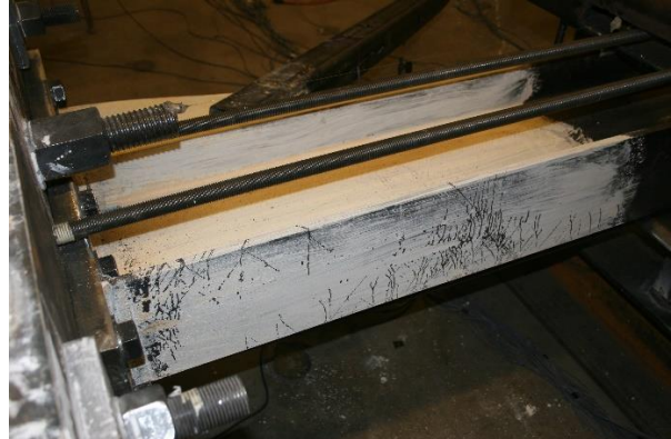
Figure 4.40 Outer Flange Yielding at Column Base (NE) 1.4% drift
