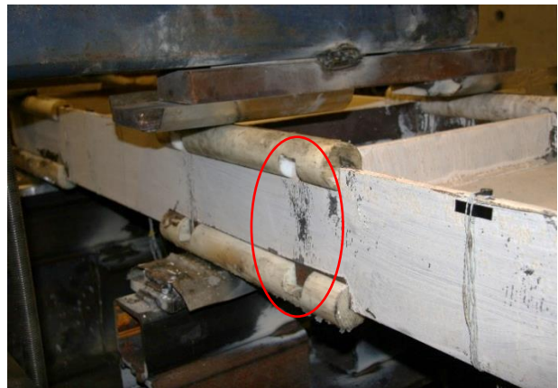
Figure 4.68 Beam yielding @ -3.2% Drift
