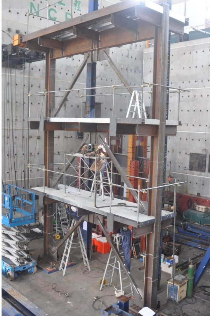
Figure 6.1 Chevron 7 overview picture (prior to testing)
