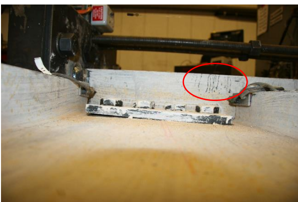
Figure 4.20 Beam end torsion @ -1.9% drift
