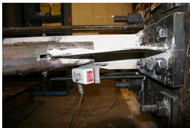
Figure 4.21 Buckling @ NE corner gusset @ +1.9%
