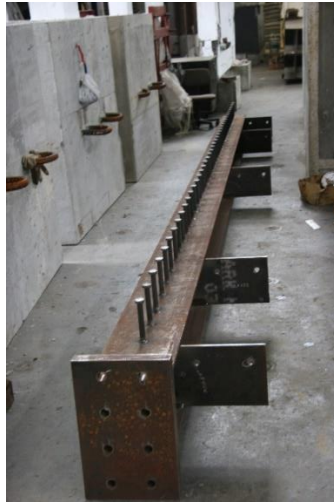
Figure 6.16 Top slab edge beam
