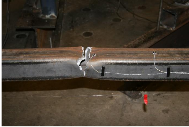
Figure 4.30 S Brace @ +3.6% drift
