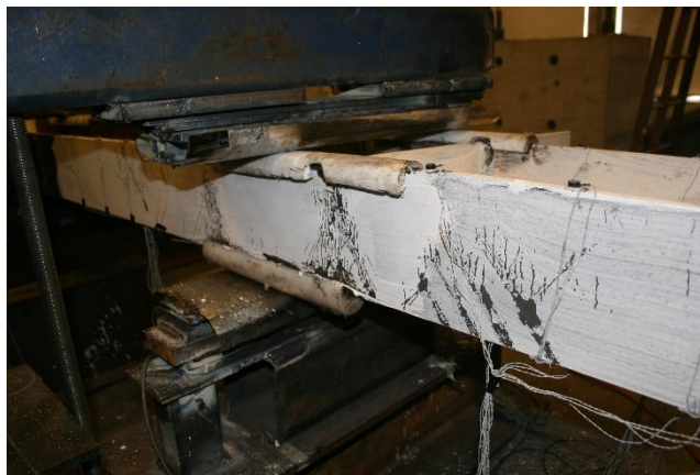
Figure 4.43 Beam Yielding Extending from Stiffeners @ 1.9%
