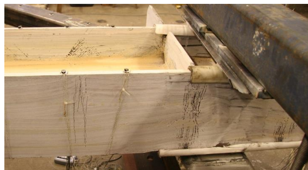
(a) Chevron 2 beam yielding
