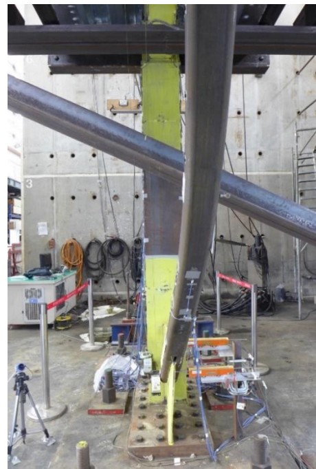
(f) 1SBr buckled at -0.45% roof drift
