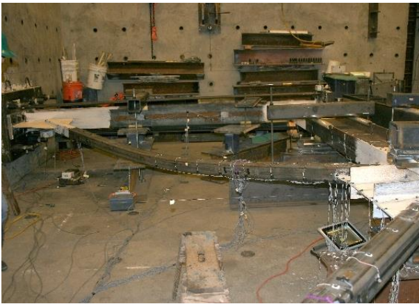
Figure 4.35 South Brace Buckling @ 0.7% drift
