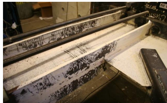
(b) Chevron 3 north column yielding
