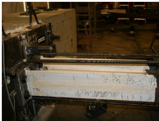
Figure 4.59 South column yielding @ 1.4% drift
