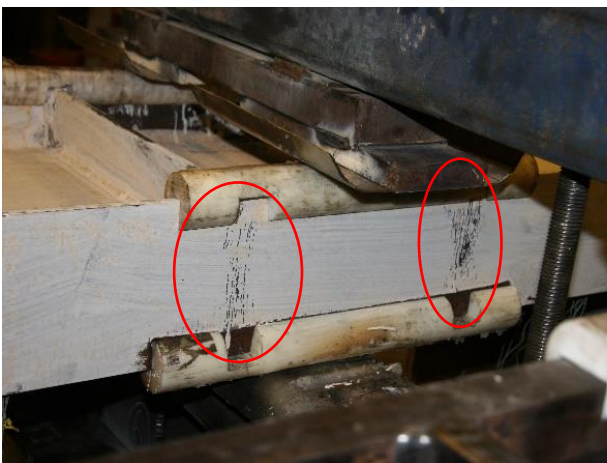
Figure 4.58 Beam OF yielding @ 1.1% drift
