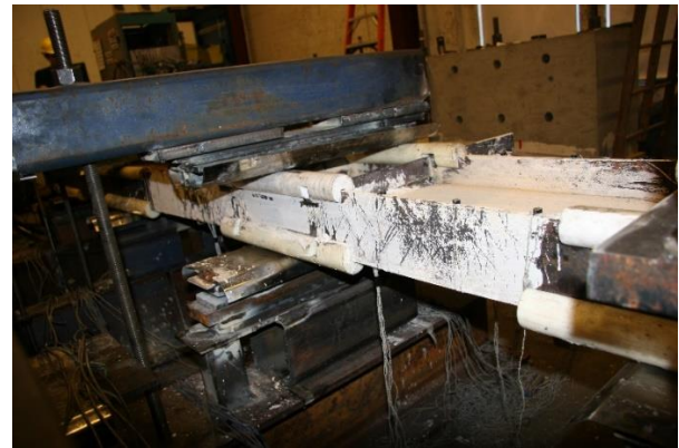
Figure 4.27 Beam yielding @ -3.0 % drift
