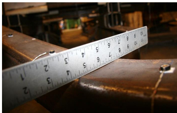
Figure 4.62 Cupping in N brace @+2.5% drift
