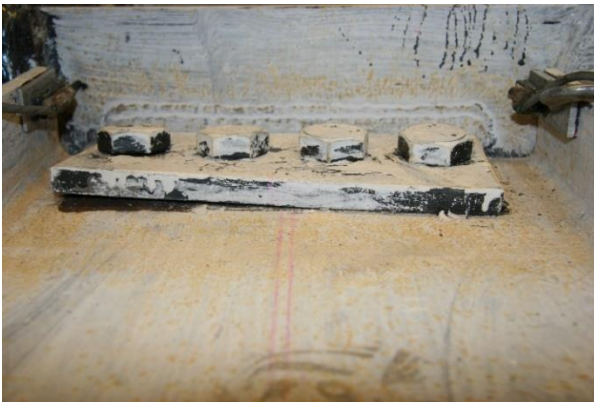
Figure 4.26 Beam end torsion @ 3.0% drift
