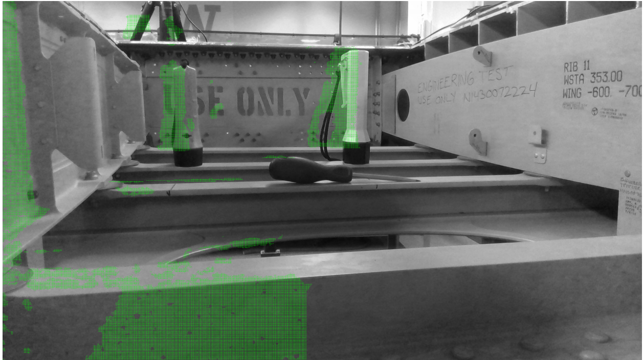
Figure 3.19: Spatial detection: points from the changed cloud in Figure 3.18 are projected back into the camera frame and the nearest pixel for each projected point is changed to green. All non-green pixels are selectively set to grayscale in post-processing to better visualize the detections.
