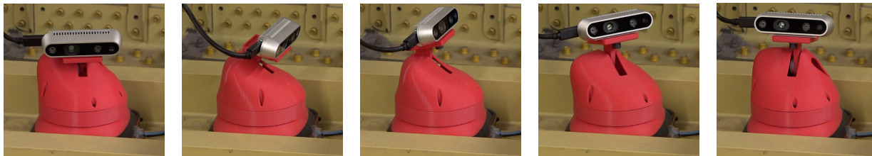
Figure 2.2: Mapping procedure: the robot moves between waypoints, collecting depth images, converting them to point clouds and transforming them into the world frame to construct a 3D map of the wing.
