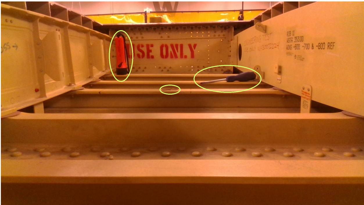
Figure 3.1: Debris placed in the wing: flashlight, key and screwdriver labeled by hand.
