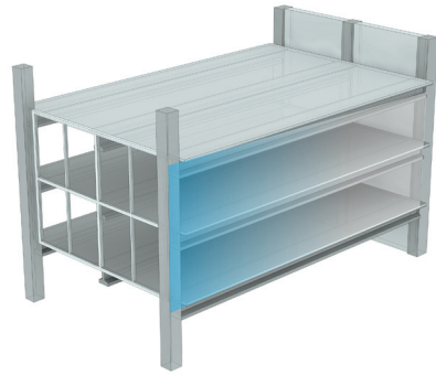
Figure 6.16a: Enclosure in the plane of the columns will allow thermal bridging through the concrete structure and make heating the new building costly.
