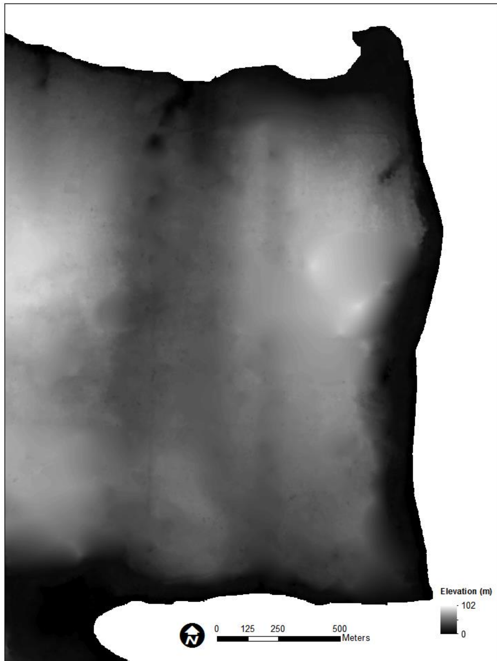
Figure 9. Digital Terrain Model of Bill Point produced using aerial photos and Agisoft PhotoScan.
