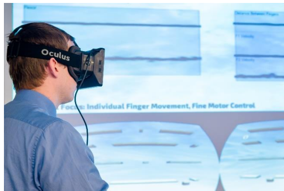
Figure 4.2.8. VR Headset used in prototype version of the vHAB system. In this example, the user is playing an early version of a pinching game using the VR headset.
