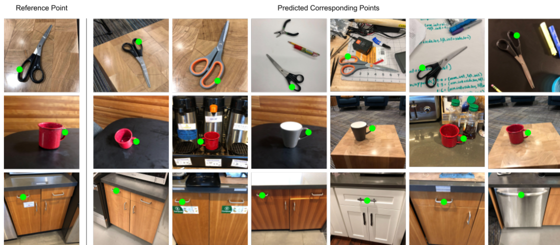
Figure 4.3: In Diffusion-PbD, features from a pre-trained Stable Diffusion [104] image model are utilized to transfer demonstrated contact points to new scenes. The examples in this figure show the effectiveness of this method at finding corresponding points in novel viewpoints, objects, and scenes. The reference points on the left are extracted from human demonstrations, and the corresponding points on the right are predicted through the use of diffusion features.
