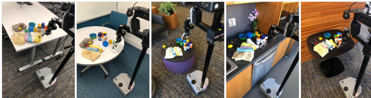
Figure 4.4: We evaluate Diffusion-PbD using a Stretch RE2 robot to perform 14 real world manipulation tasks across 5 visually distinct environments. We show that this approach is effective for single-shot imitation of a wide range of manipulation tasks and generalizes to novel viewpoints, objects, and scenes.
