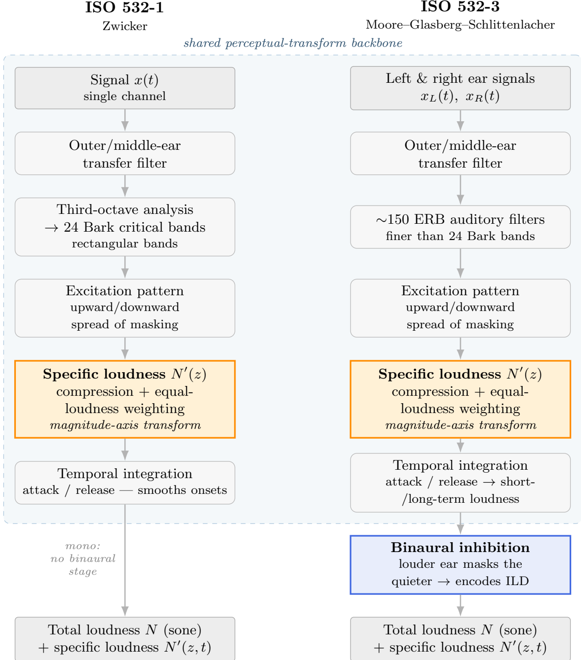
Figure 2.2: High-level block diagrams of the two loudness models. Both share a perceptual-transform backbone (dashed box): an outer/middle-ear filter, an auditory filterbank, an excitation pattern that models spread of masking, a compressive specific-loudness transform (highlighted), and temporal integration. ISO 532-1 (Zwicker) uses third-octave analysis mapped to 24 rectangular Bark bands; ISO 532-3 (Moore–Glasberg–Schlittenlacher) uses ~150 ERB roex filters and adds a binaural-inhibition stage in which the louder ear masks the quieter, encoding the interaural level difference. The highlighted specific-loudness block is the magnitude-axis transform central to this thesis.
