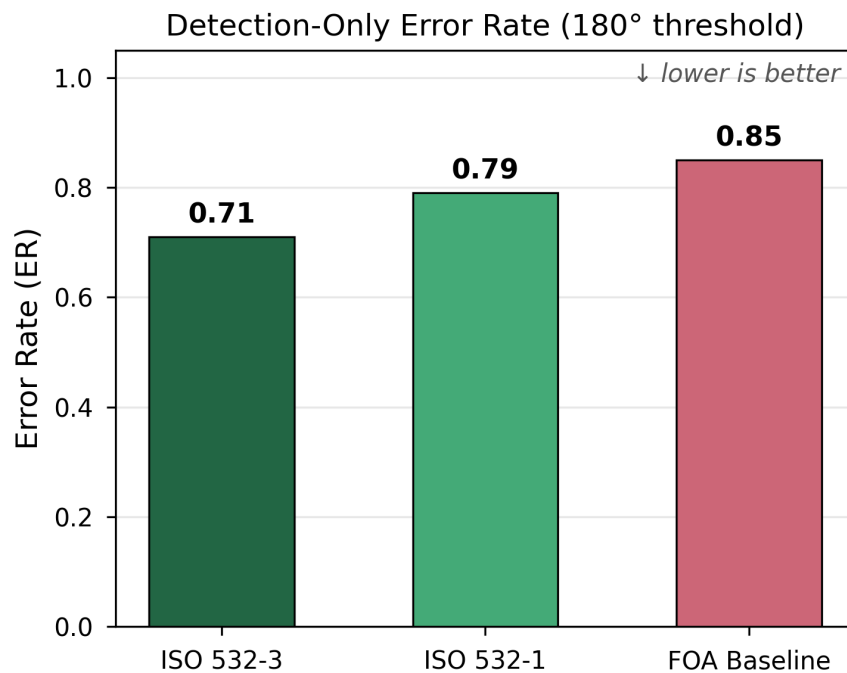
Figure 4.5: Error rate at the 180° threshold (detection-only, no location constraint). The ISO 532-3 loudness model attains the lowest error rate—fewer total errors, consistent with fewer false alarms—using only 2 channels versus 4 for FOA. As the F-scores in Table 4.4 show, this reflects more conservative detection rather than higher recall.
