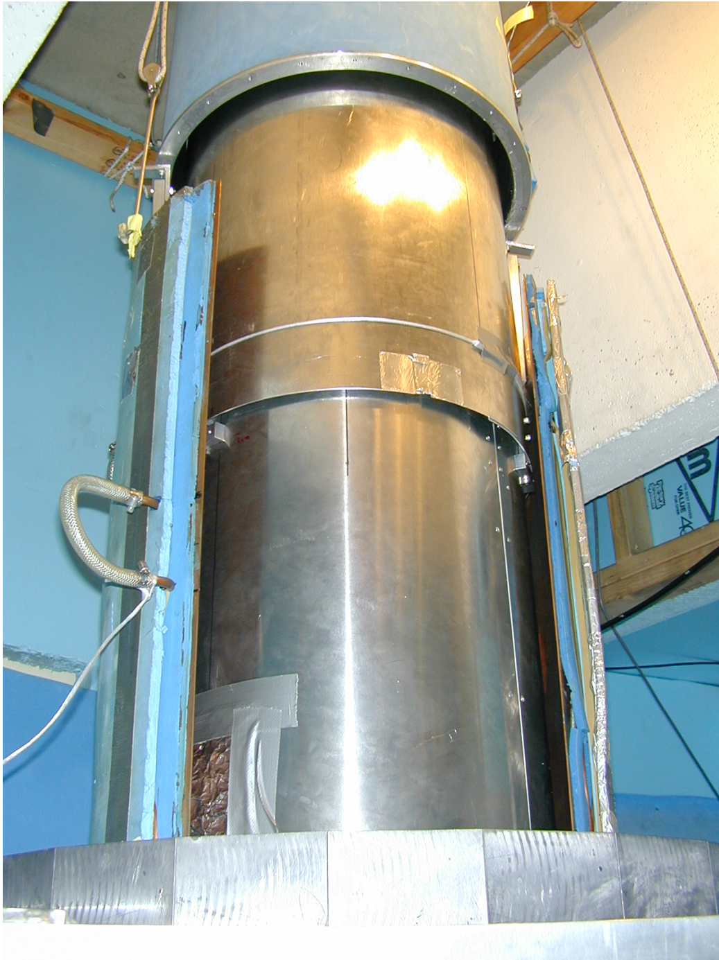
Figure 7.8: Independent temperature control of two cylindrical panels placed near the apparatus creates a large horizontal temperature difference that we use to determine the twist induced by temperature gradients.
