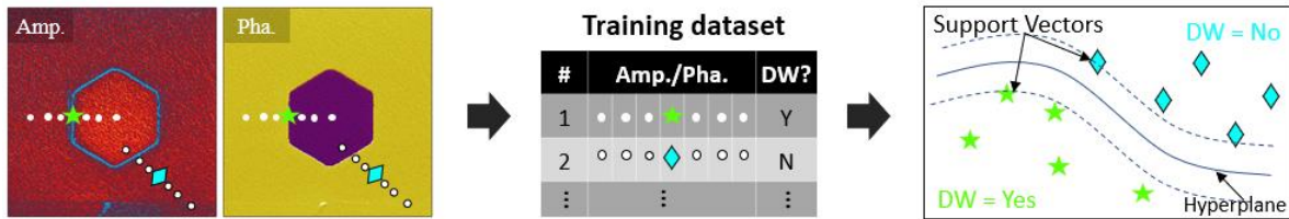
Figure 5.5. Schematics of training dataset using PFM mappings of \text{LiNbO}_3 and the corresponding classification of ferroelectric DWs.
