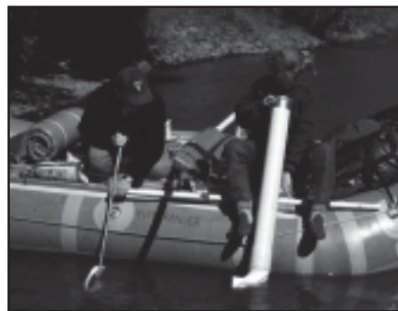
Ashley uses the horizontal Secchi disc to measure light availability.
