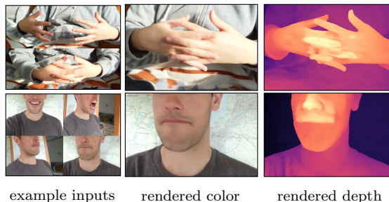
Figure 3.20: Topological changes break our method. The recovered geometry can be incorrect despite looking good from some viewpoints.
