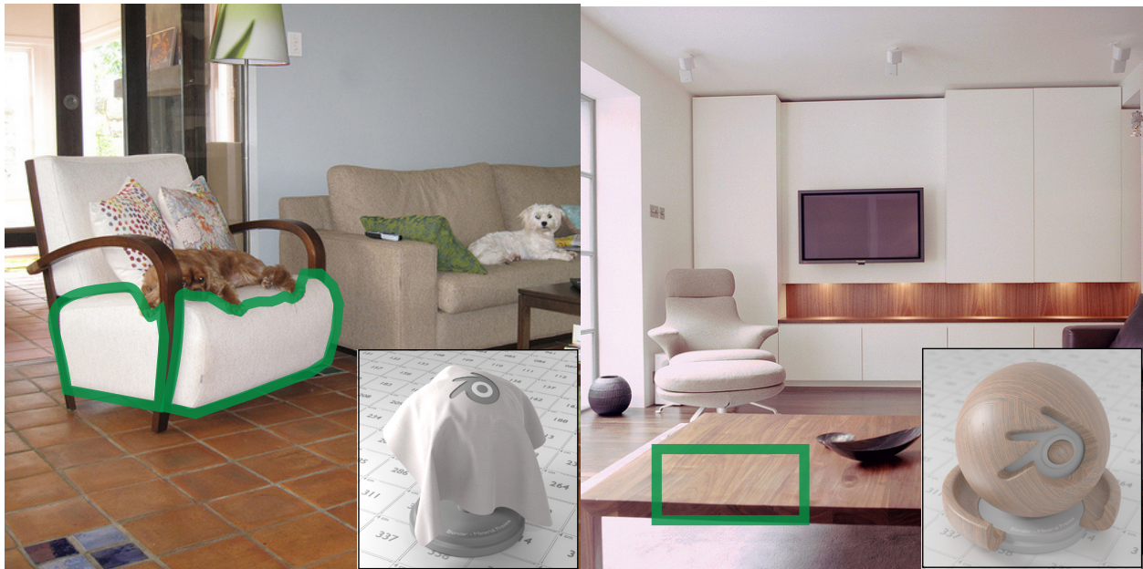
Figure 5.14: Without any additional training, our network is able to make reasonable predictions on natural images. The input image and colored outline for the segmentation mask is shown on the left. The top BRDF retrieval for each segment are shown on the right.
