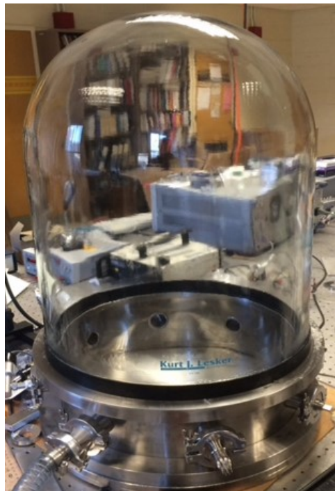
Figure 3.4: Vacuum enclosure to house rotation stage
