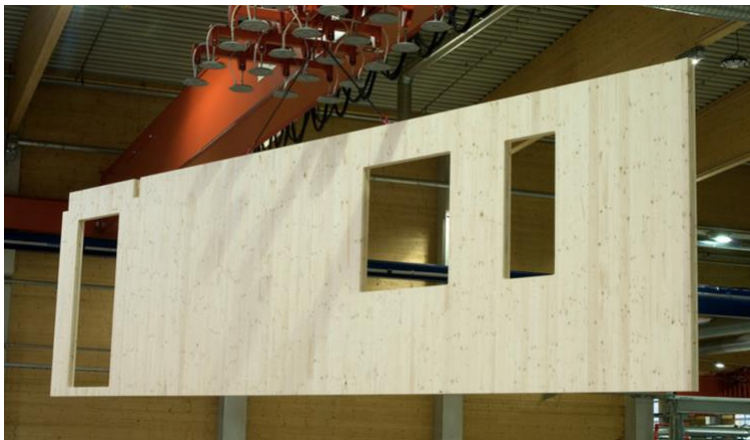
Figure 6: CLT under Construction at Stora Enso (Jones et al., 2016)
