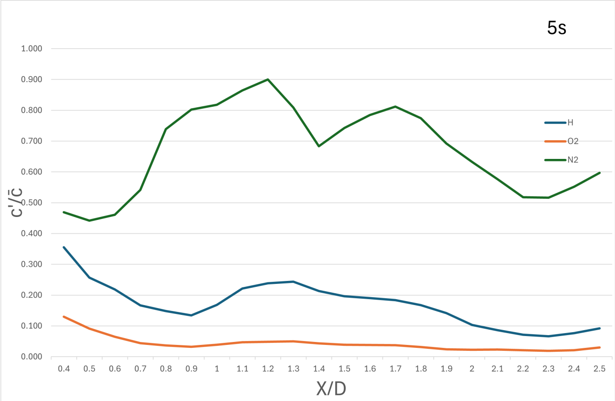
Figure 5.18: Concentration fluctuation ratio at downstream cross sections 5s into simulation
