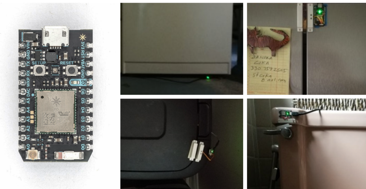
Figure 4.10. Photon with sensors on the washing machine, fridge, garbage can, and toilet
