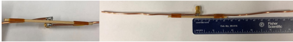
Figure 4.2: Initial antenna design, consisting of two copper wires (13 cm each), one connected to the center pin of an SMA connector and one connected to ground.
