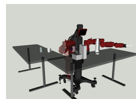
Figure 4.4: Example problem from the 7-DOF Baxter manipulator dataset, where the right arm must move from below the table to above.
