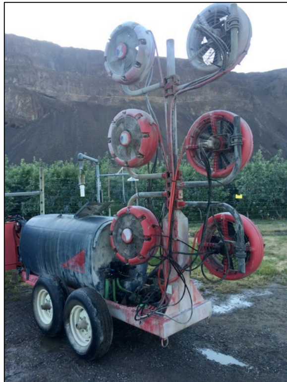
Figure 12. Multi-Headed Fan Tower (MFT) Sprayer
