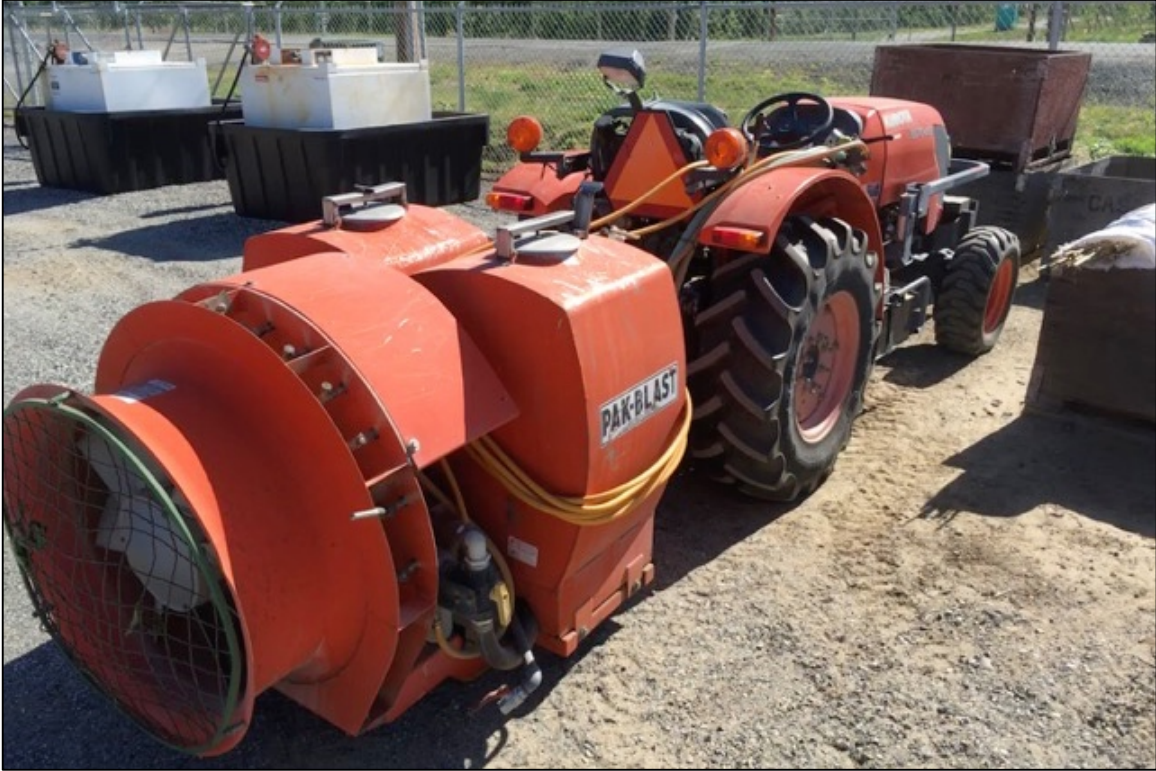
Figure 11. Traditional Axial Fan Airblast (AFA) Sprayer
