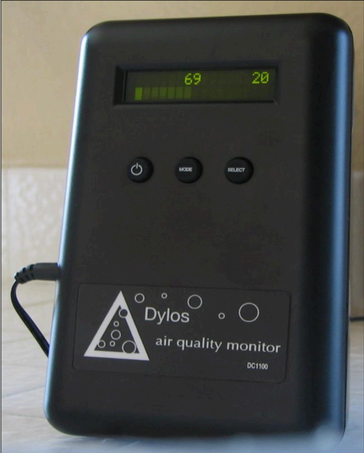
Figure 8. Dylos DC1100 Optical Real-Time Particle Monitor
