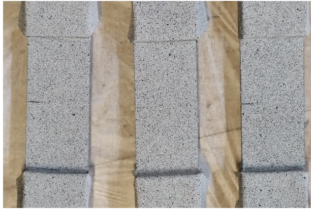
Figure 2.4: Example of DIC speckle pattern applied to specimens Speckle pattern shown is typical, but specimens are not from this work
