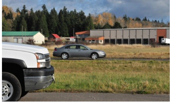
Figure 4: Road testing on a closed course (a de-commissioned airport runway). The experimented-on car, with our driver wearing a helmet, is in the background; the chase car is in the foreground. Photo courtesy of Mike Haslip.
