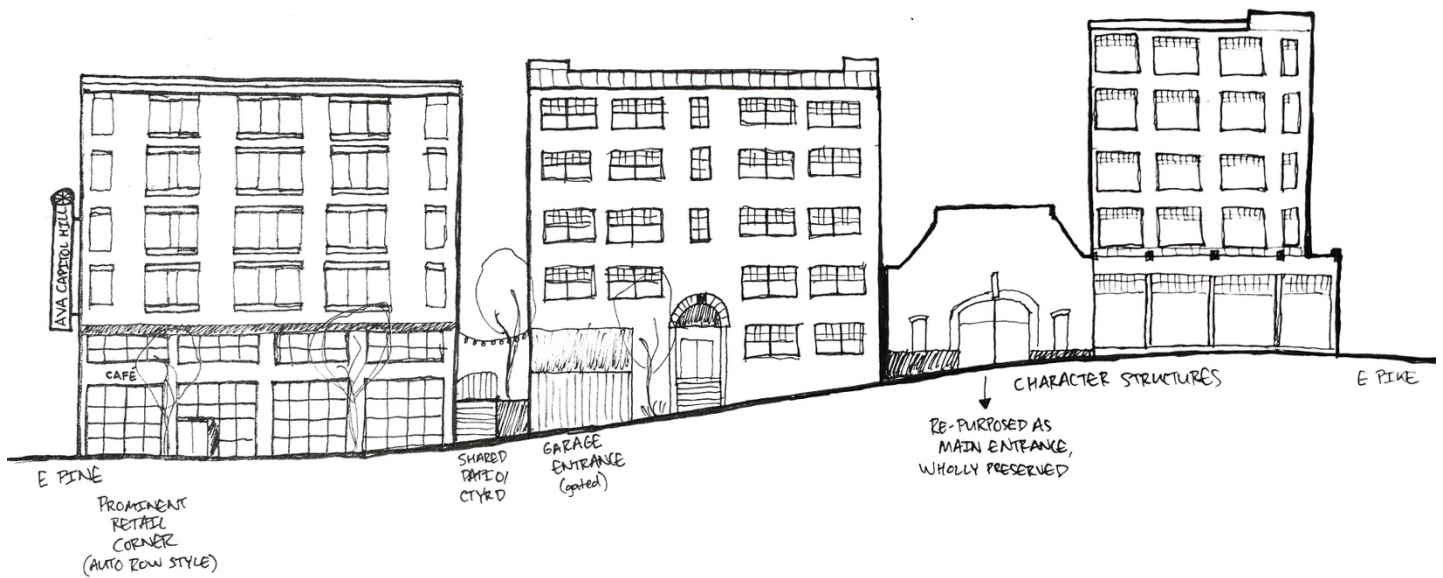
Figure 28 (above): Sketch of what the AVA project might have looked like with a form-based code applied, from the same perspective as Figure 23. Note the three separate masses with Auto Row architectural features as opposed to a mass that takes up the whole block, and the complete preservation of the most iconic character structure. Source: Scott Cutler.
