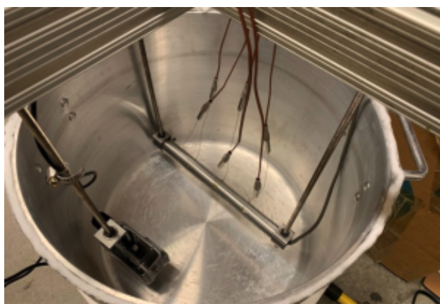
Figure 2.3: Horizontally mounted grooved cylinder.
