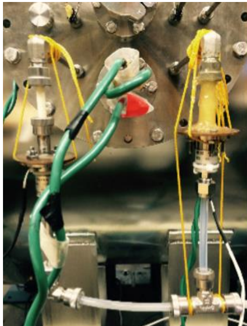
Figure 3.6: Gas Puff Valves (Left) and IGBT Controller Circuit (Right)
