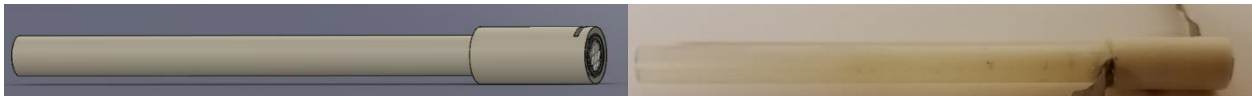
Figure 3.7: Pre-ionization source: design (Left) and actual (Right) using ceramic alumina tubes for electrical isolation
