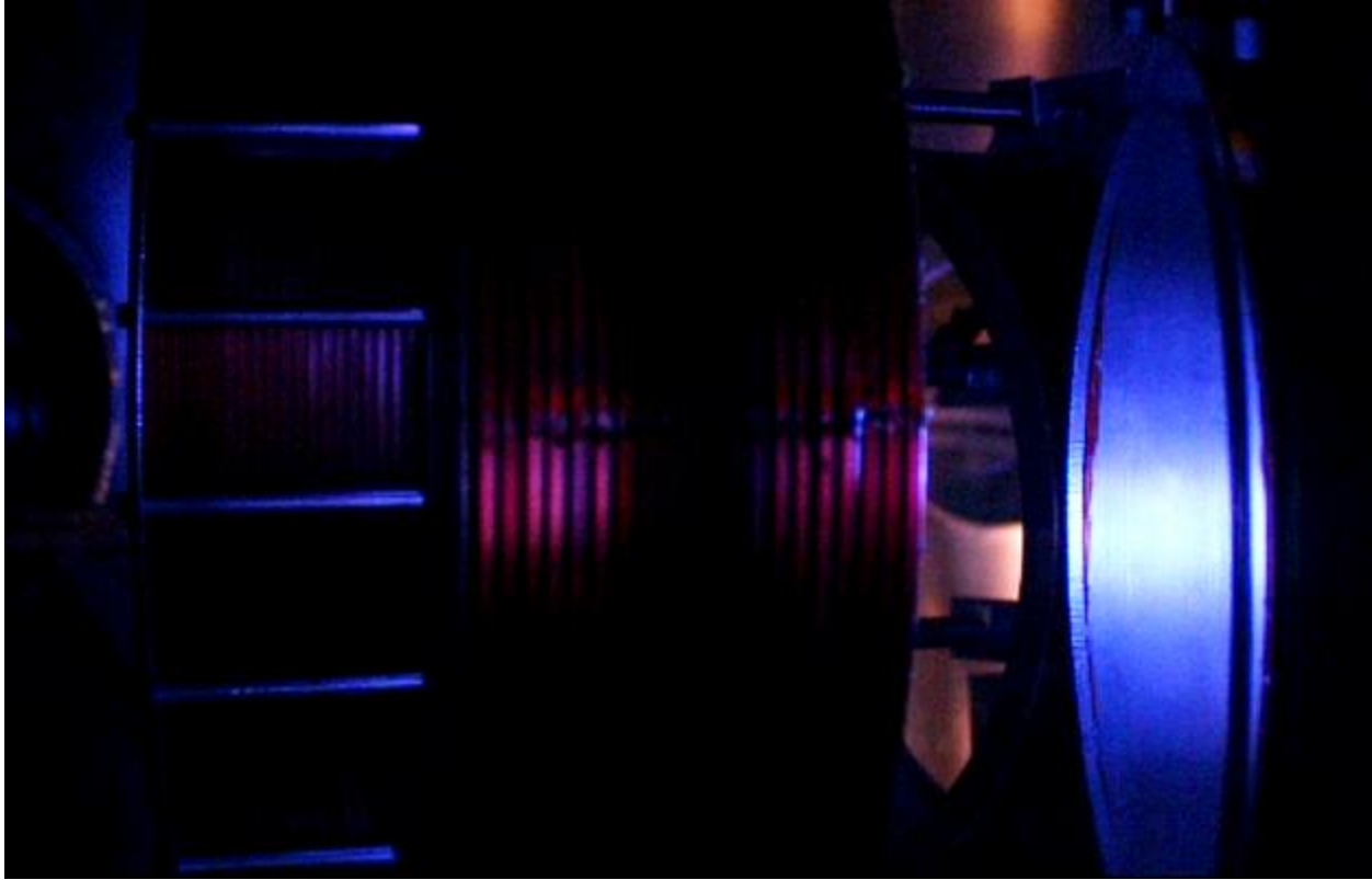
Figure 6.2: Initial plume visualization of the HPH cluster in the variant 3-magnetic flux conserving configuration.
