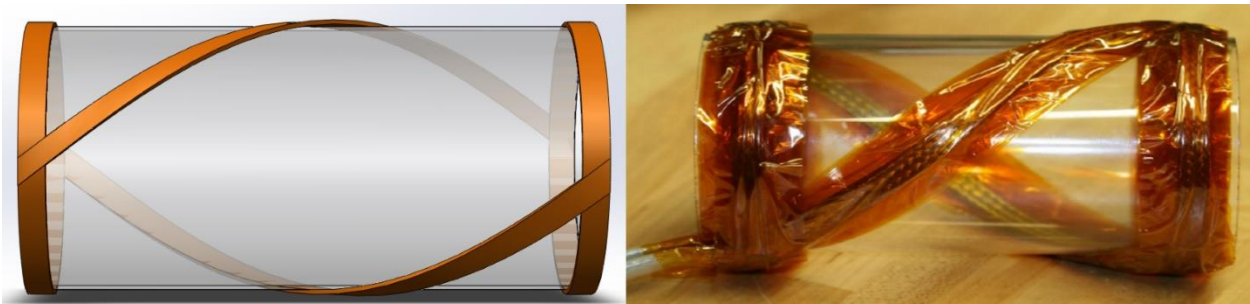
Figure 3.9: Left-handed Nagoya Type III helical antenna, (Left) design and (Right) actual
