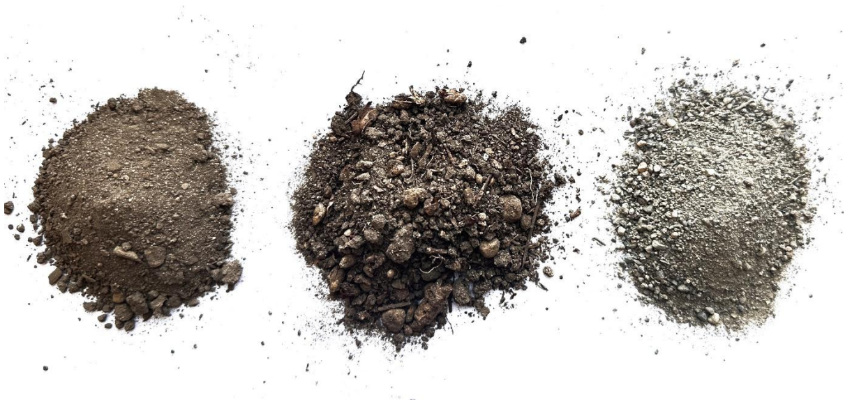
Figure 10. Three soil types used in experiments: (left) loamy soil, (center) organic-rich garden soil, and (right) sandy soil. Each differs in texture, composition, and moisture retention properties.
