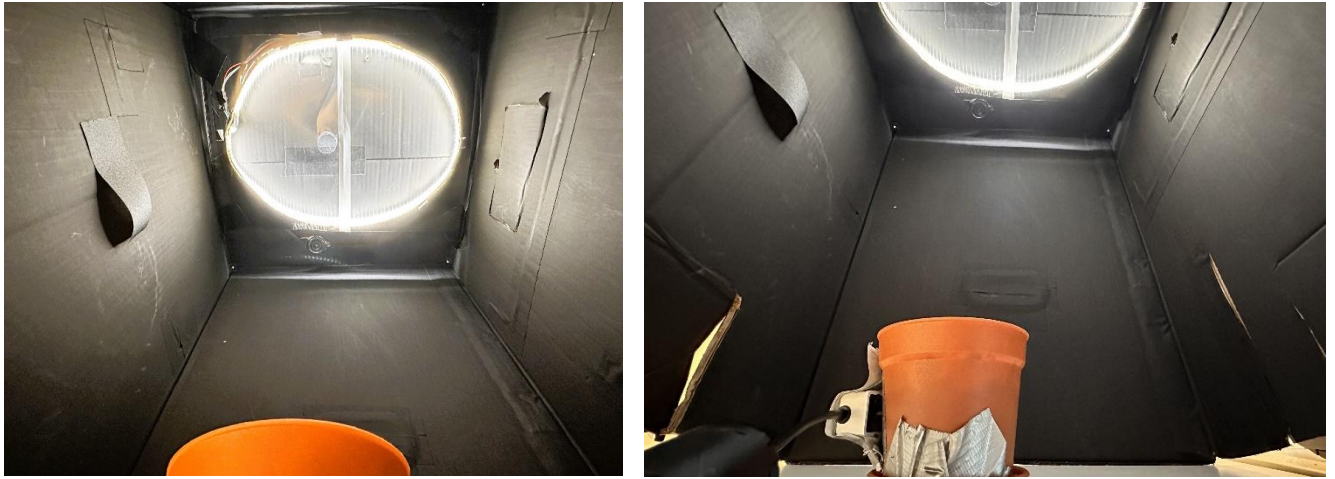
Figure 8. Experimental setup showing a soil sample placed inside a box, illuminated by a ring light with a linear polarizer. A camera is angled through a top opening to capture polarized reflectance near Brewster's angle.
