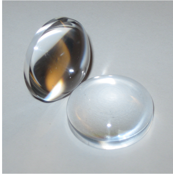
Figure 5.20: Polished aspherical acrylic (vertical) and polycarbonate (horizontal) lenses.
