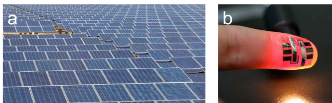
Figure 1-1 (a) Conventional rigid solar cell devices. (b) Modern conformable infrared photodetector device.
