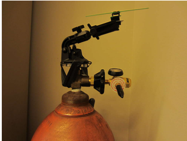
Figure 2.11: The WISPCam , mounted on an industrial gas cylinder, monitors a pressure gauge.
