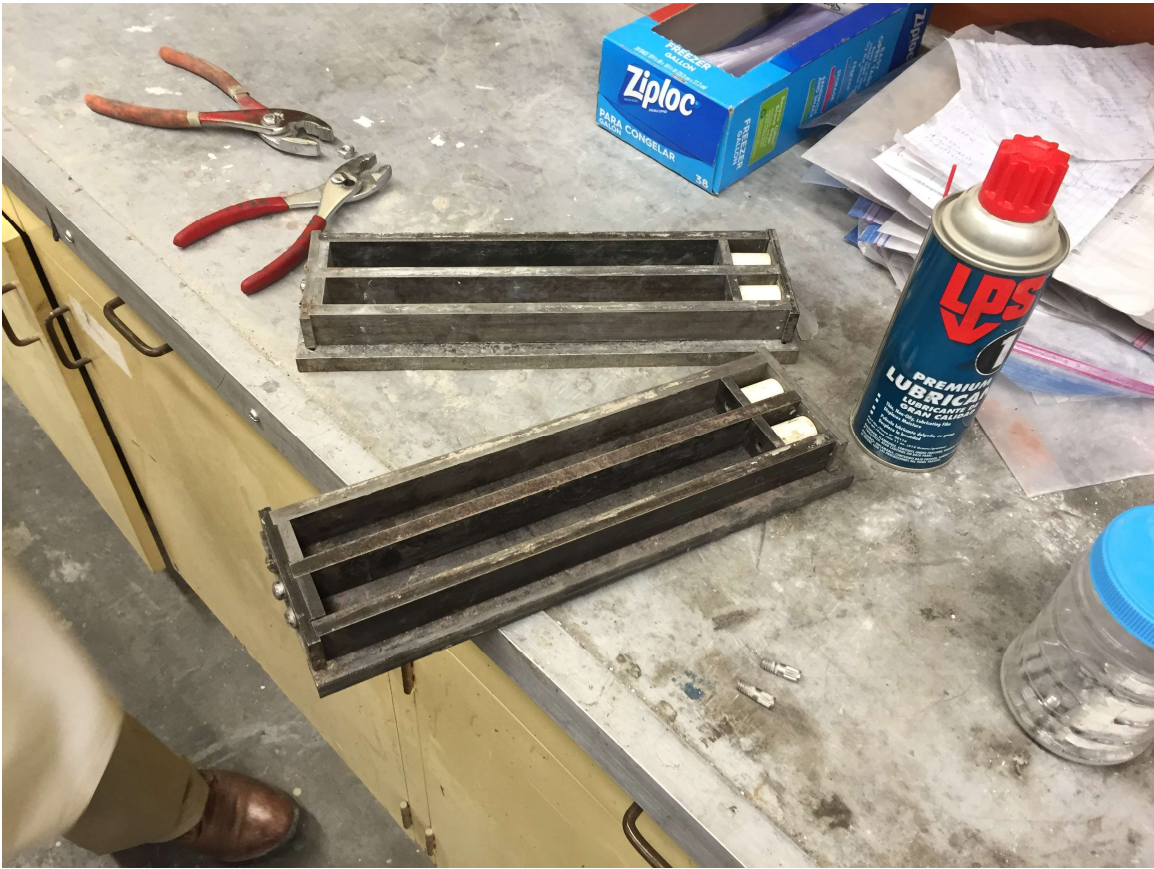
Figure B-2. Mortar molds were used to make the mortar bars. A triplicate subset of mortar bars for each ASTM C1260 trial was mixed into three of the four available molds. Prior to curing, the concrete was casted in the molds, then covered and stored in room temperature for a period of 24 hours.
