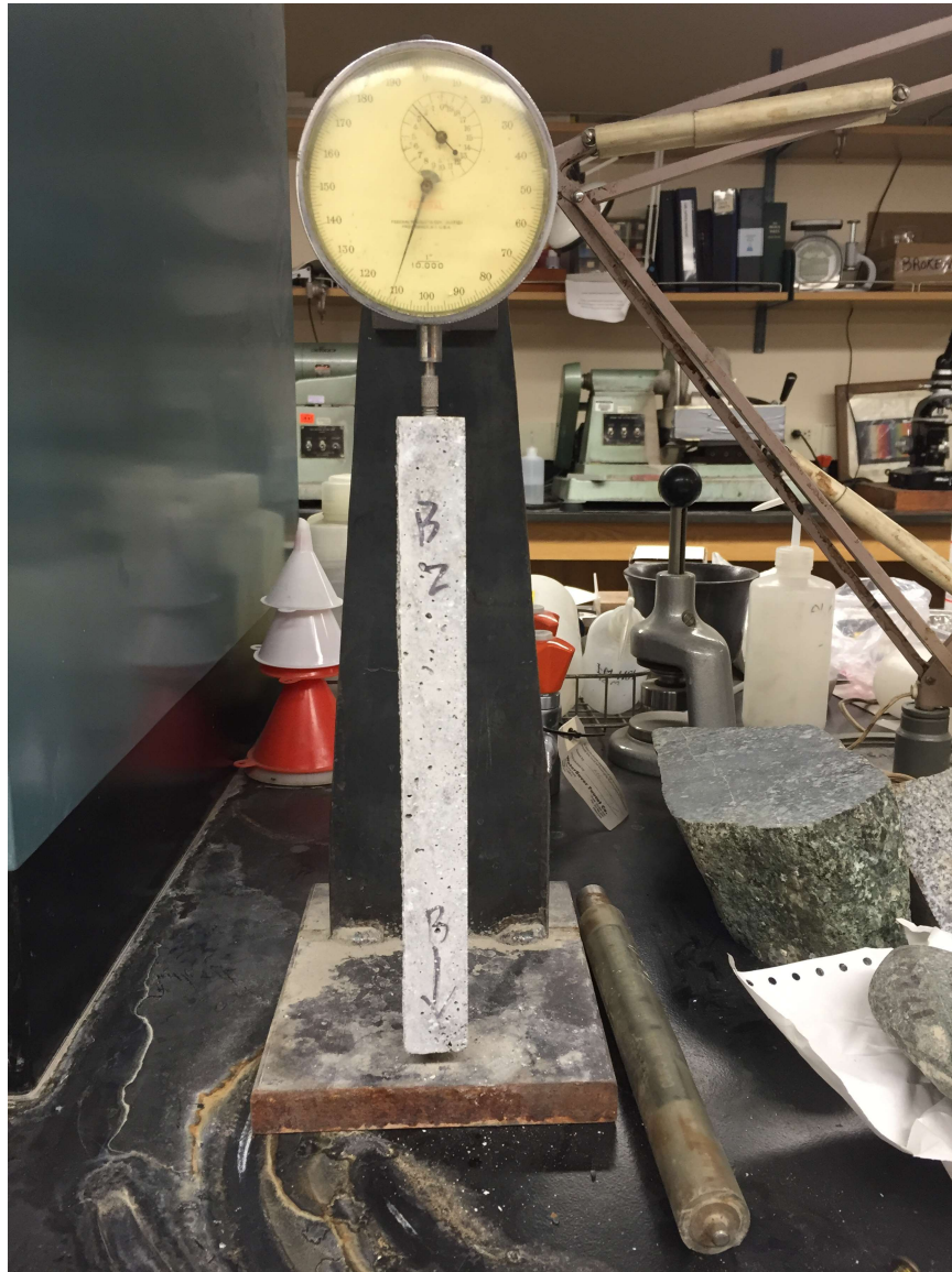
Figure B-3. The dial comparator used for the ASTM C1260 trials was accurate within 0.0001 inches. A reference bar (right of comparator), was used to zero the comparatory readings prior to each mortar bar measurement. The mortar bars were placed upright so that both gauge studs are on the comparator stage.
