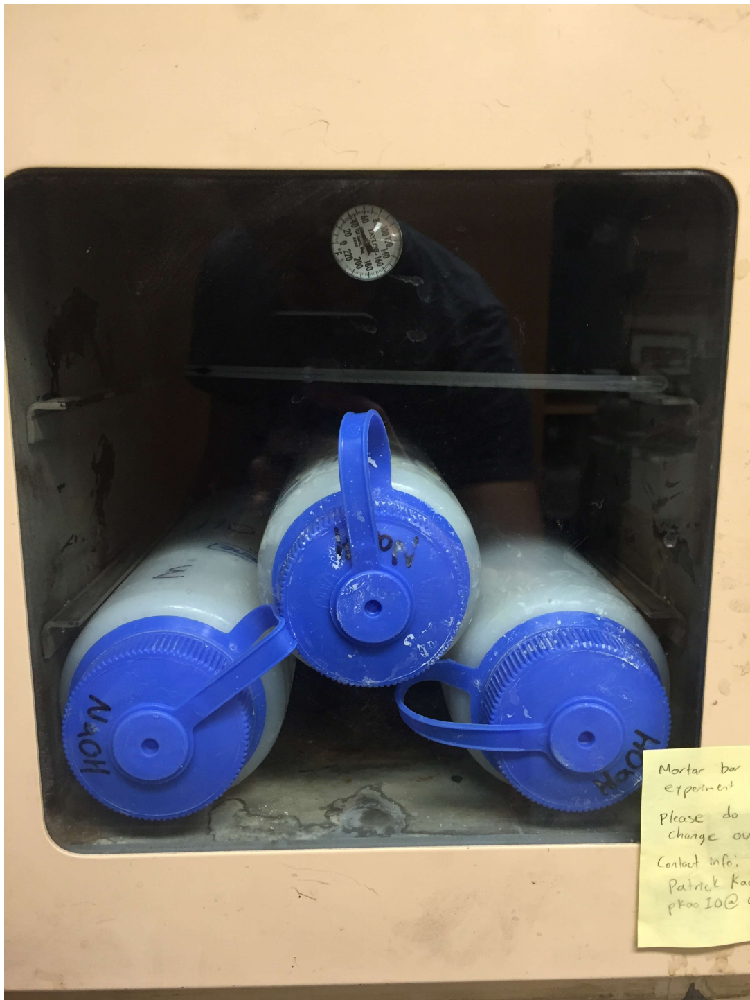
Photo B-4. Two Fisher Scientific ovens (Model 48) were used to maintain the temperature of specimens during the 14 day tests. High density polyethylene containers each contained 1L NaOH solution and one mortar bar specimen. These containers were placed horizontally, to ensure full submersion of solution.
