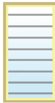
5. Timber frame with clear glass and iron guard rails
