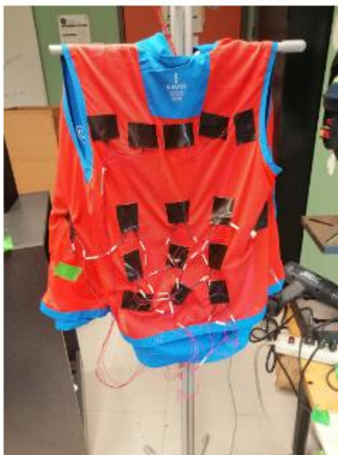
Figure 21: Image of actuators inside a haptic vest. These are meant to vibrate when specific stimuli are perceived. Jonathan Lane-Smith, “Haptic Interfaces for Musical Notation and Expression,” 47.
