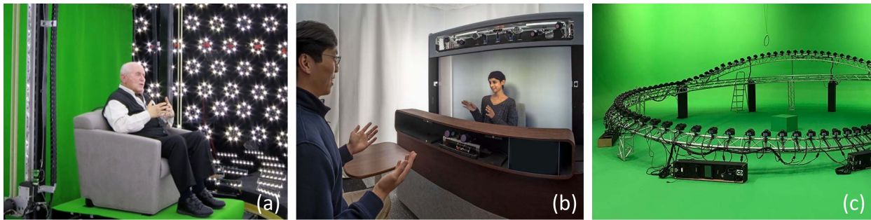
Figure 1.1: Three projects that lift the visual storytelling to 3D. (a) “New Dimensions in Testimony” [167] create an interactive 3D holographic interview experience; (b) “Starline” [83] aims to achieve an immersive remote video communication; (c) creating the bullet-time scene [181] in the movie “The Matrix” typically requires multiple slow-motion cameras placed around the action in a circle. Photo credits to University of Southern California, Google, and New World Designs.
