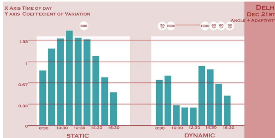
Fig A.4: Initial Results: COV with Position Changes, Delhi, Case 800A + E
