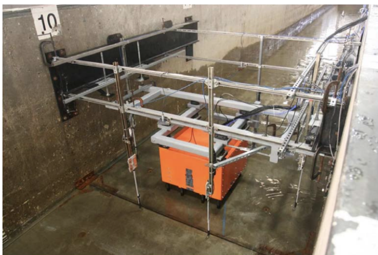
Figure 1.2: Test set-up at NHERI Wave Flume in 2017 (from Winter et al. (2020) ).
