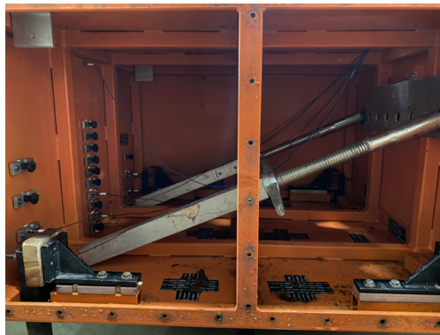
(c) Internal structure of test structure; threaded rods and HSS provide stiffness from front bottom edge of box to the streamwise load cells.
