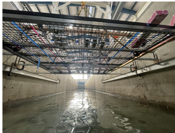
Figure 2.11: Electromagnetic/drop frame from underneath.
