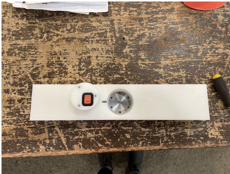
Figure 2.9: Debris with accelerometer compartment removed and Xsens DOT accelerometer.
