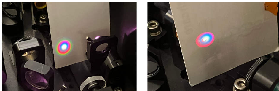
Figure 4.18. Left: Example of good white light generation through a sapphire. (The camera has slightly amplified the red ring around the white core from what the human eye can see.) Right: Example of white light generation through a burned sapphire.
