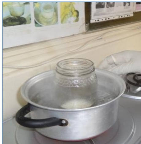
Figure 41: Low cost, low-tech flash heat pasteurization being used at a human milk bank. A milk jar, without a lid, is placed in a pan of water, which is then heated. When water reaches a rolling boil, milk reaches a temperature high enough to deactivate contaminants like HIV and other pathogens. Photo credit: King Edward Hospital, Durban, South Africa.
