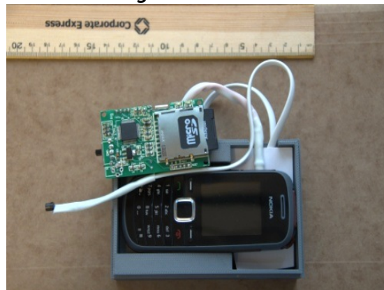
Figure 9: FoneAstra with a temperature sensor (at the end of the white cable) and connected to a Nokia mobile phone. The ensemble, packaged in the gray box visible around the phone, has final dimensions of 12cm X 8cm X 5cm.
