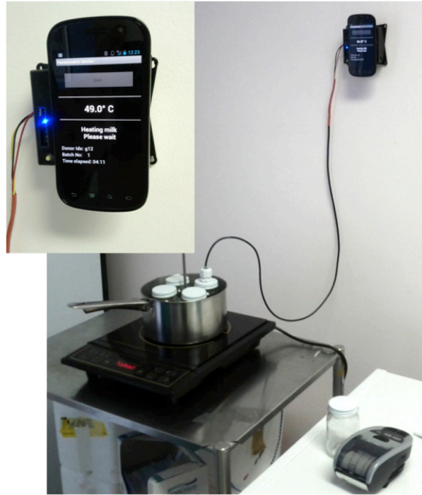
Figure 16: The third and final version of the milk pasteurization system installed at a human milk bank in South Africa. It uses the FoneAstra 3.0 board to interface the temperature sensor to Android over Bluetooth. FoneAstra is inside a black enclosure that is mounted on the wall, and the Android phone is mounted on the enclosure. The inset shows a close-up view of the ensemble. Cf. Chapter 5 for more details about the human milk banking project. Photo credit: Paarl Hospital, Cape Town, South Africa.
