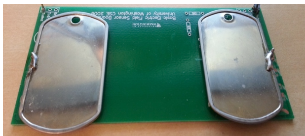
Figure 81: An early prototype of FoneAstra's single-lead EKG daughterboard. EKG data is sent from FoneAstra to a co-located Android over Bluetooth when a subject places their thumbs (or fingers) on the two steel plates. Software (currently under development) on the Android processes the sensor data to detect anomalies in the EKG.
