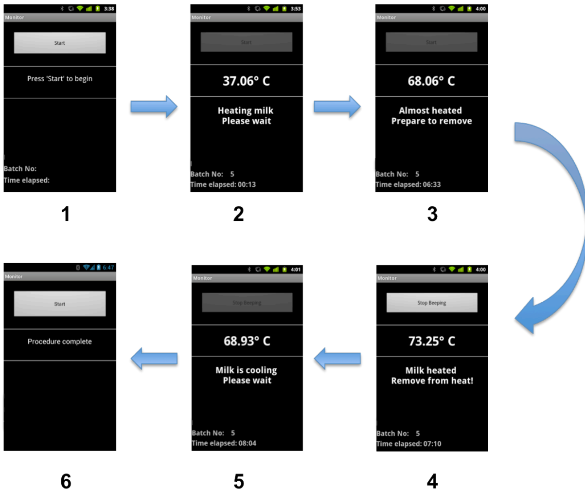
Figure 46: Screenshots of the Android application that guides the user through the pasteurization process. (1) User places water and milk jars in the water-bath and turns the stove on. Clicking the “Start” button on the app starts the pasteurization monitoring process. (2) A unique batch ID is generated for the procedure. Rising temperature is displayed on the screen along with the time elapsed. (3) Phone beeps twice to alert user at 5°C before the high temperature threshold of 73°C is reached, and the visual indicator changes accordingly. (4) The visual indicator changes at 73°C and the phone starts beeping continuously until the user removes the jars from the water-bath. (5) Beeping stops, and the visual indicator changes to indicate cooling when app detects a drop in temperature. (6) Procedure is complete when temperature drops to 25°C.
