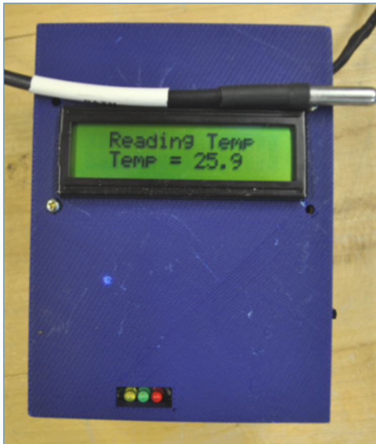
Figure 44: Pasteurization monitor V1: The mobile phone and FoneAstra are inside the blue enclosure. FoneAstra was enhanced with an LCD, water-proof temperature sensor, and an audio buzzer.
