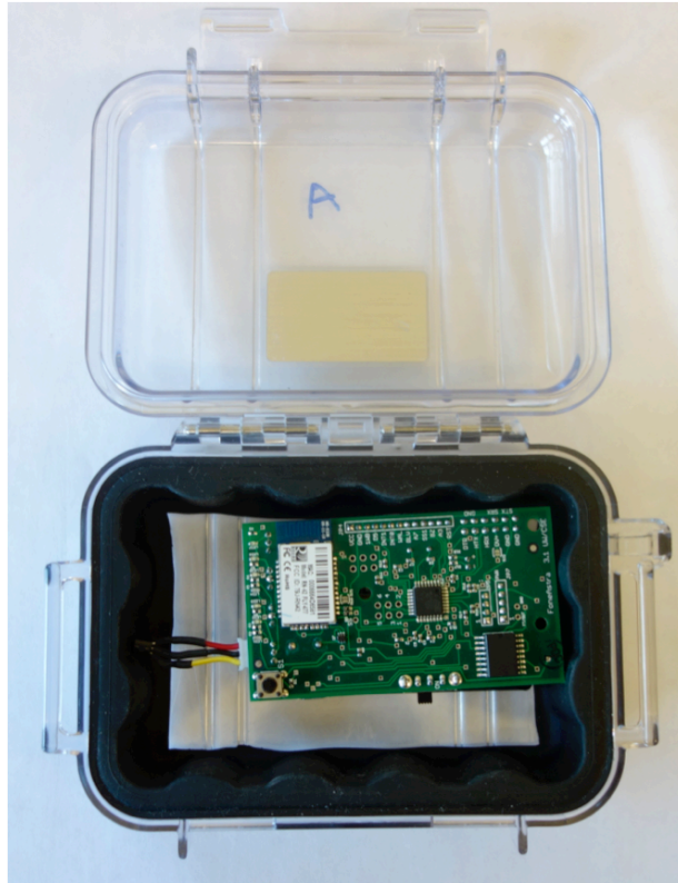
Figure 38: A FoneAstra 3.0 board with its battery (which is not visible because it is under the board) placed inside a waterproof Pelican case. The three wires protruding from the left side of the board are for the temperature sensor that is plugged into the board. This ensemble was placed inside a Styrofoam box that contained temperature-sensitive medical supplies (along with cooling gel packs to maintain a low temperature) and was used to monitor the box's internal temperature while it was in transit, being shipped from California to Port Au Prince, Haiti.
