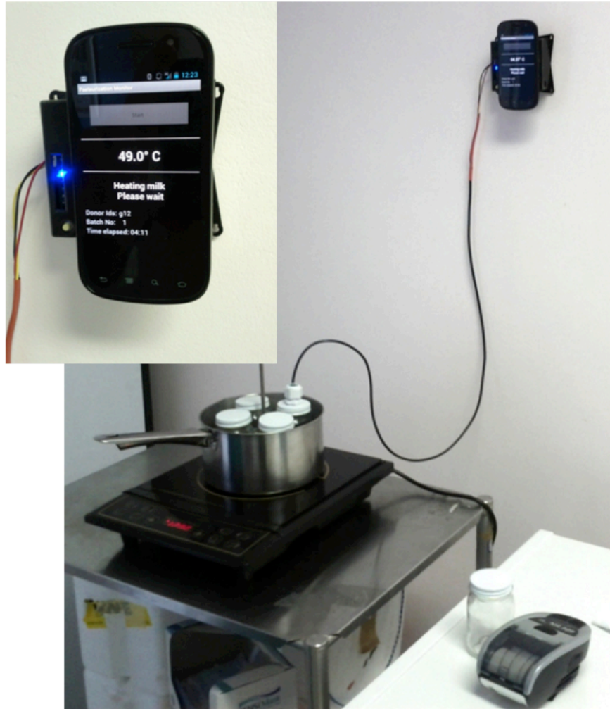
Figure 49: Pasteurization monitor V3 installed at a human milk bank in South Africa. It uses the FoneAstra 3.0 board (cf. Section 2.3) to interface the temperature sensor to Android over Bluetooth. FoneAstra is inside a black enclosure mounted on the wall, and the Android phone is mounted on the enclosure. The inset shows a close up view of the ensemble. The rest of the set up (e.g., stand, pan, stove etc.) is the same as in V2. Photo credit: Paarl Hospital, Cape Town, South Africa.
