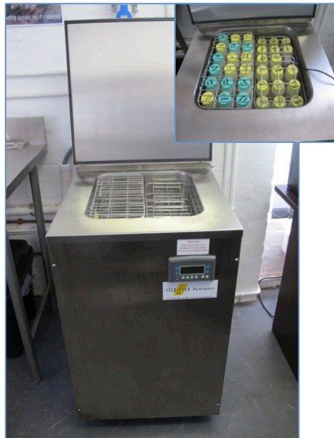
Figure 40: A high-end commercial pasteurizer. It provides temperature monitoring and archiving on a computer via a temperature probe that is connected to the computer. Milk bottles placed in the pasteurizer are shown in the inset. Photo credit: iThemba Letu transition home, Durban, South Africa.
