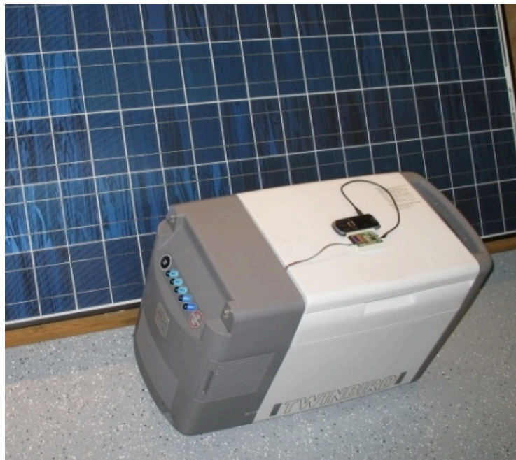
Figure 26: A solar powered cold box enhanced with temperature monitoring. FoneAstra and the connected Nokia 1661 mobile phone are placed on top of the cold box. The temperature sensor connected to FoneAstra is placed inside the cold box. Photo credit: PATH, Seattle, USA.
