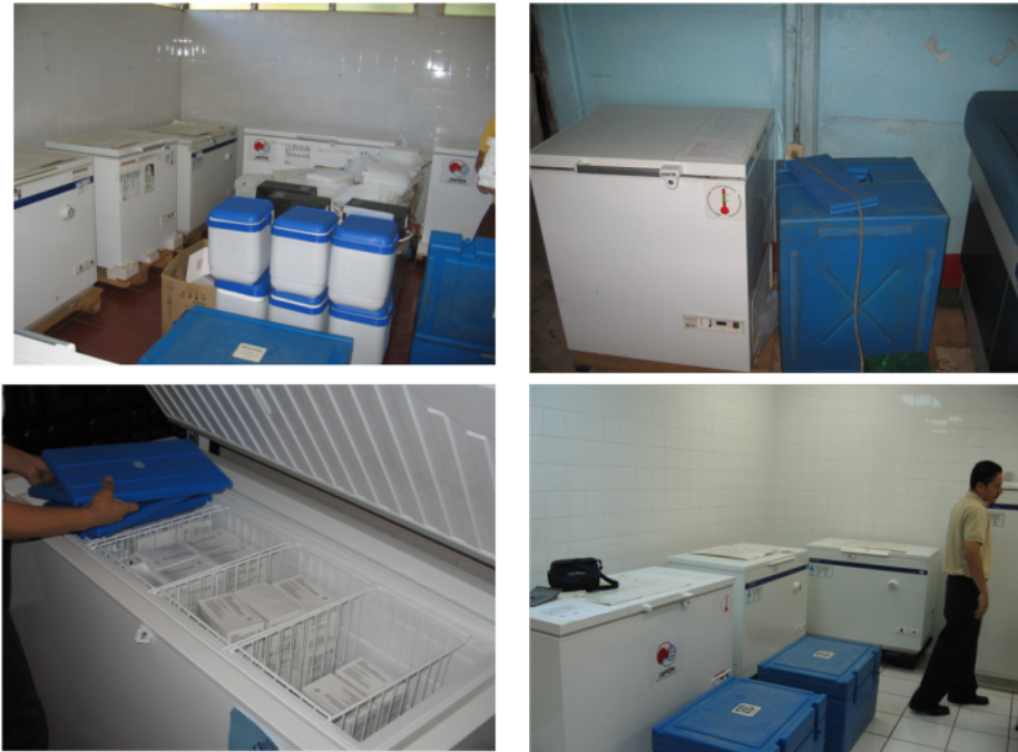
Figure 21: Refrigerators and cold boxes used for vaccine storage and transportation. Photo credit: Prof. Richard Anderson, UW, Seattle, USA.
