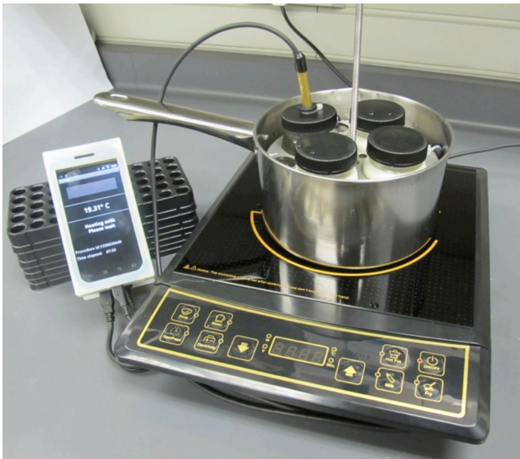
Figure 48: Pasteurization monitor V2. A stand holds 4 glass jars. The temperature probe connected to the mobile phone is secured on the jar containing water; the other jars contain milk. The stand with jars containing liquid is placed in a water-bath that gets heated on an induction stove. The white enclosure on the left side of the picture hosts the mobile phone and the USB Bridge that connects the probe to the phone. Photo credit: Pediatrics Lab, University of KwaZulu-Natal, Durban, South Africa.
