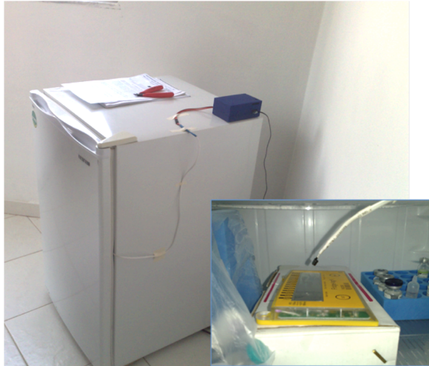
Figure 31: FoneAstra deployed at a health center in Tirana. Note the box on the top back-right corner of the household fridge and the wire going down to the door and through the insulating lining. The inset shows the temperature sensor hanging inside the fridge, just above a FridgeTag for comparing temperature readings from both devices. Photo credit: Ministry of Health, Albania.
