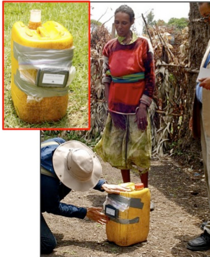
Figure 11: Researcher attaching time-use sensor to a water container. The lady is the primary water collector for the household. Photo credit: Yuta Masuda, UW, Seattle, USA.
