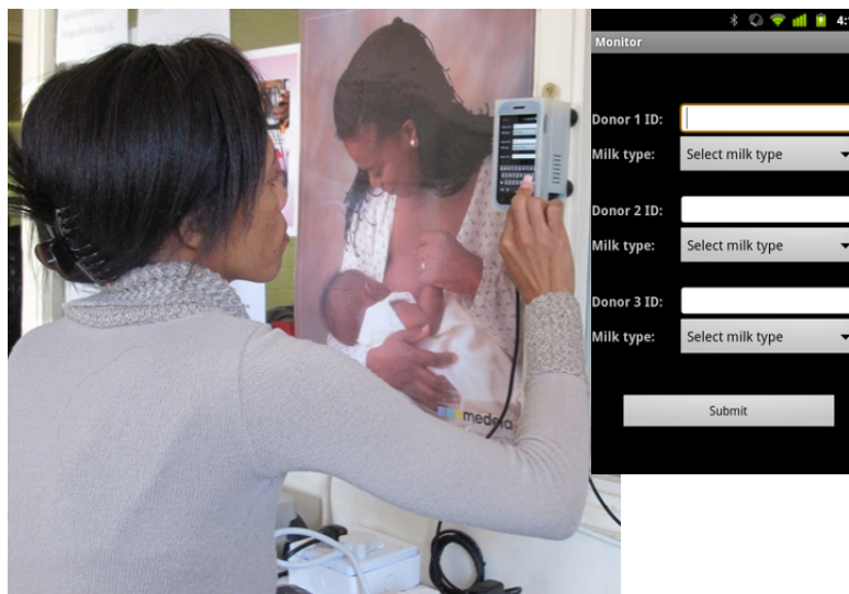
Figure 57: Pasteurization monitor V2 at the Neonate ICU of King Edward Hospital. The milk bank technician is entering donor information in the mobile app. The inset is a screenshot of the Activity that lets the technician enter information. Photo credit: King Edward Hospital, Durban, South Africa.
