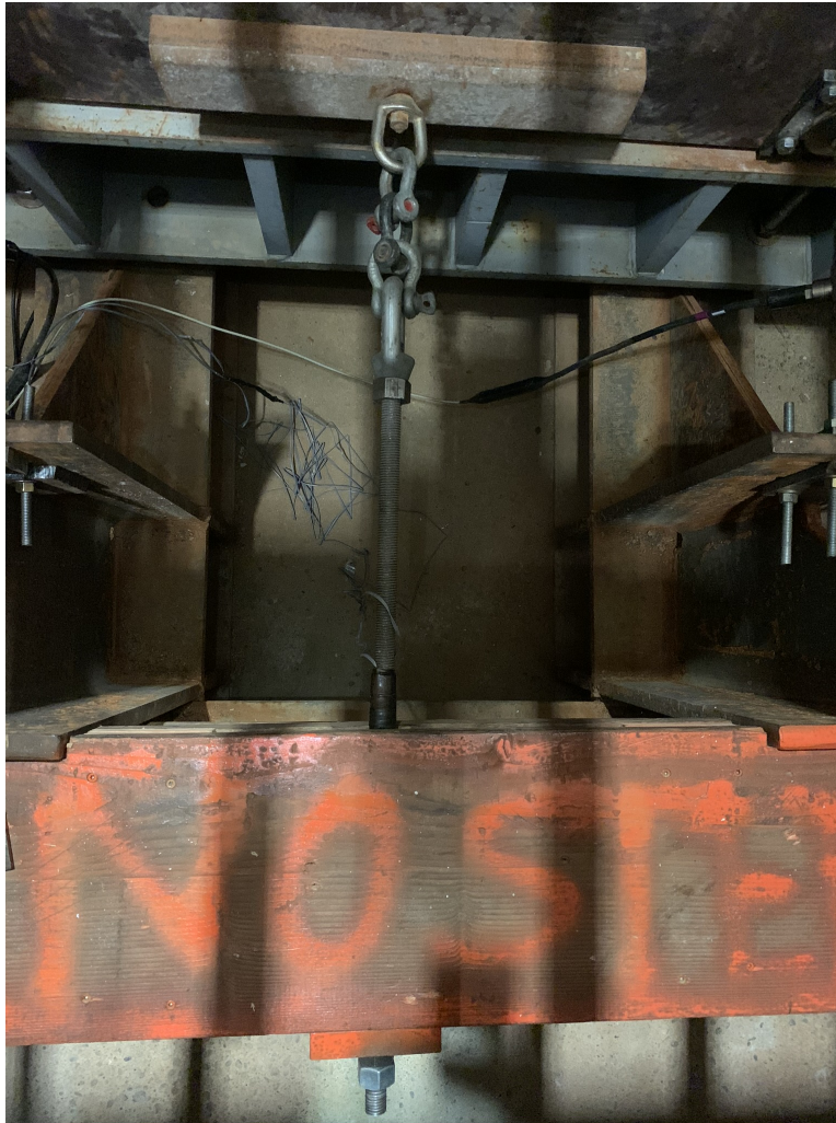
Figure 4.10: Threaded rod connects the back of the specimen to the reaction frame. The threads on the rod and nuts allow the streamwise load cells to be compressed to a specified preload. At the mid point of the rod, the threads are ground down, so a strain gauge can be applied.
