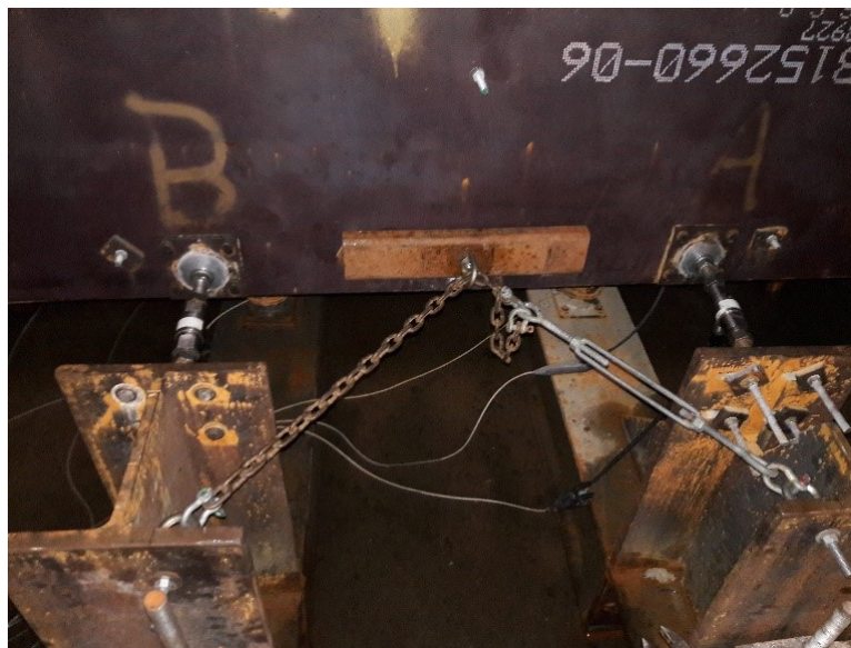
Figure C.3: Load Cell Pretensioning Chain and Turnbuckle
