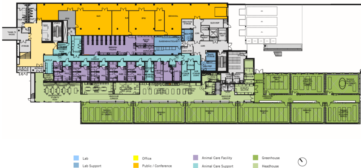
Figure 10: Basement 1 Floor Plan of the LSB Project indicating the location of the various labs and green houses on the building
