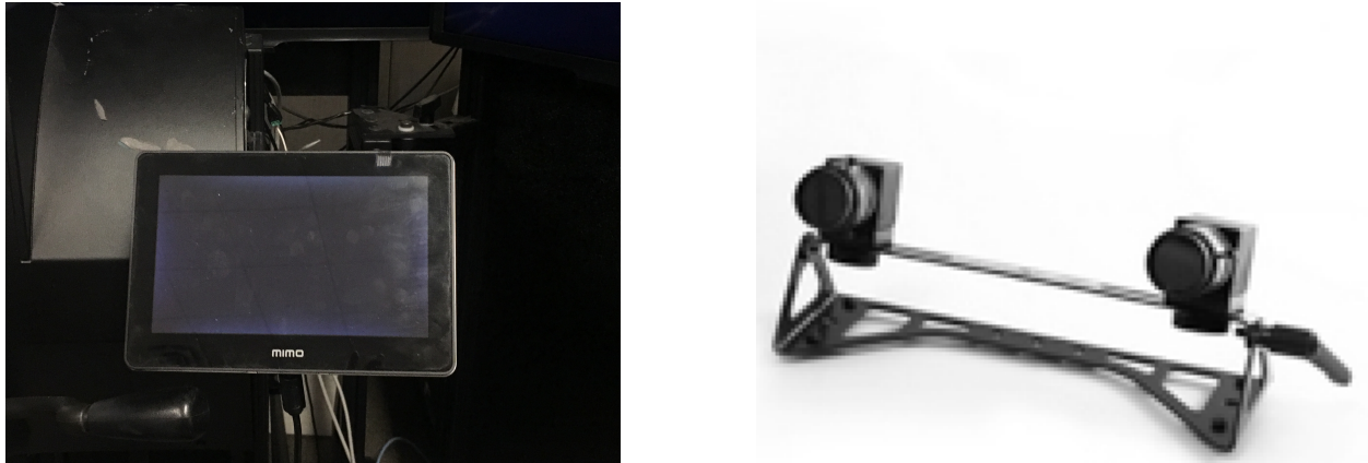
Figure 3.7: The mini touchscreen (left) is used in the secondary task; the faceLAB™ eye tracker system (right) is used for eye movement and glance behavior data collection
