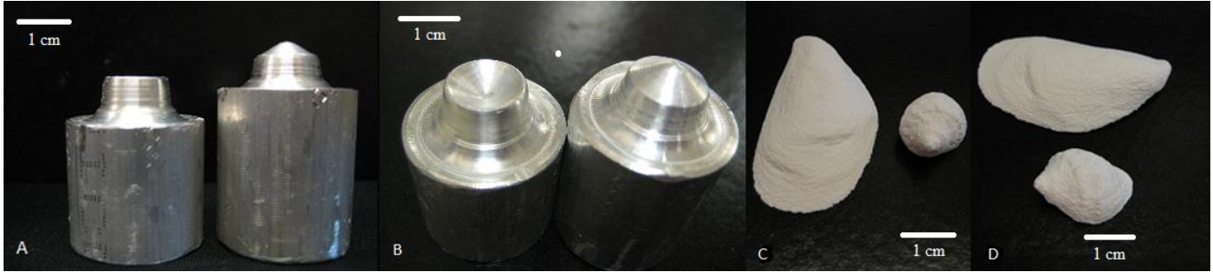
Figure 1. (A) Side and (B) top views of aluminum cupped and pointy teeth. (C) Top and (D) lateral views of printed mussel and snail shells.
