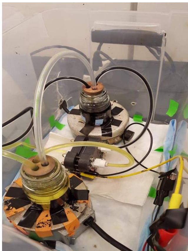
Figure 2.9. Image of full-cell RFB during charge-discharge operation.
