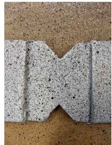
(d) Speckle painted specimen for DIC analysis
