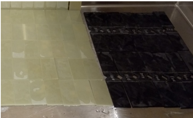
(c) Sanded, cleaned specimens and tab tiles before bonding
