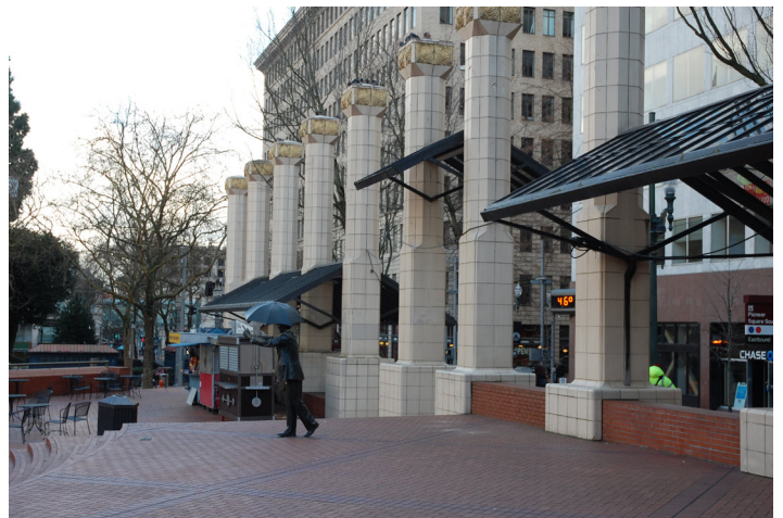
Figure 14 Large columns may block visibility
