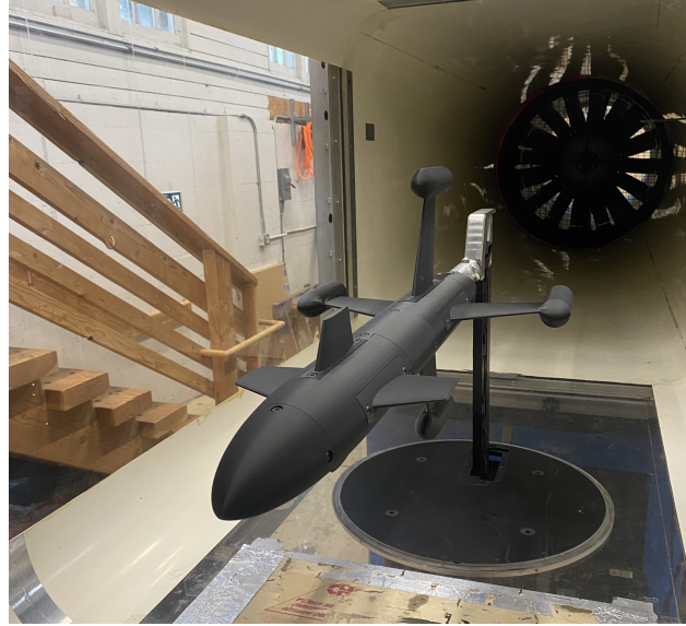
Figure 3.3: Wind tunnel configuration model mounted on the sting balance
