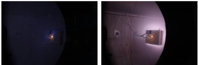
Figure 2.7: Phase 2 testing displayed that when the magnet was turned on (right) a magnetoshell would form and expand about the injected gas. Left shows the magnet off for comparison [12].
