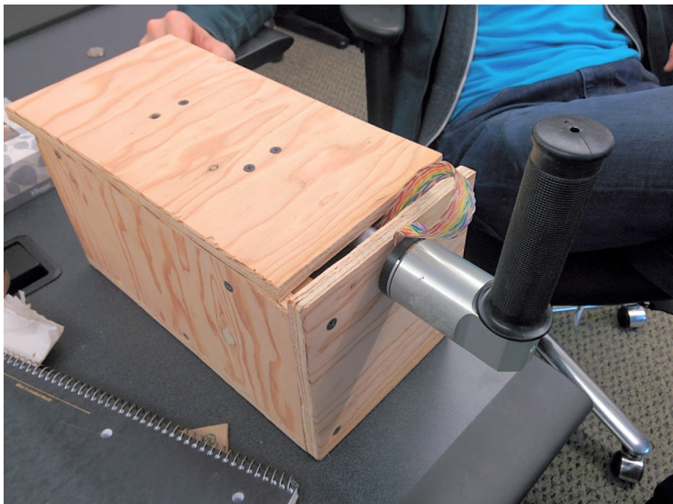
Figure 3.1: Image of an instrumented assisted walker load cell from AMTI used in this experimental data acquisition.
