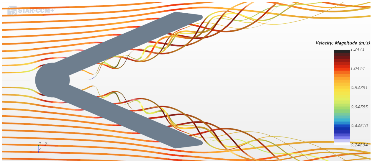
Figure 4.8: Streamlines around RDDP. Streamlines are originating from points on a section that passes through the center of RDDP.
