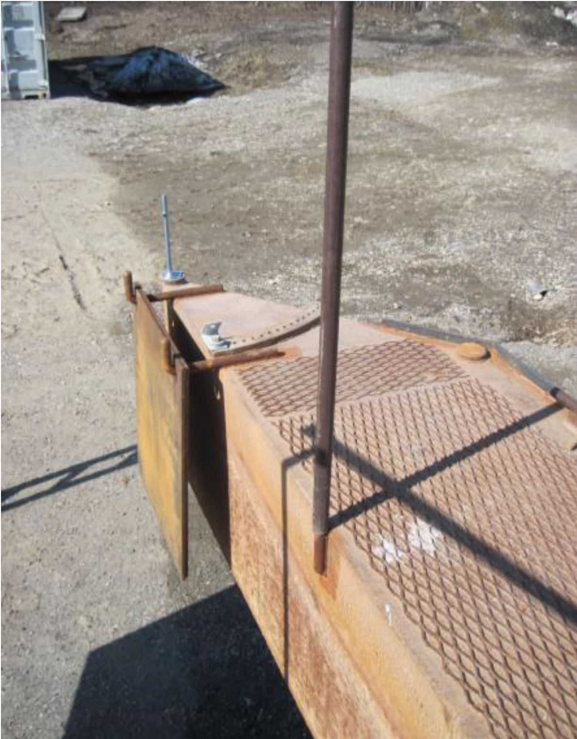
Figure 2.3: RDDP Ballast plates [13].
