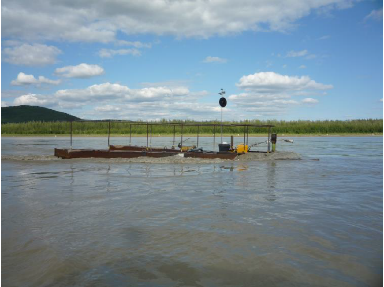
Figure 2.2: RDDP nose pitched down due to high river velocity before installing the ballast plates[13].
