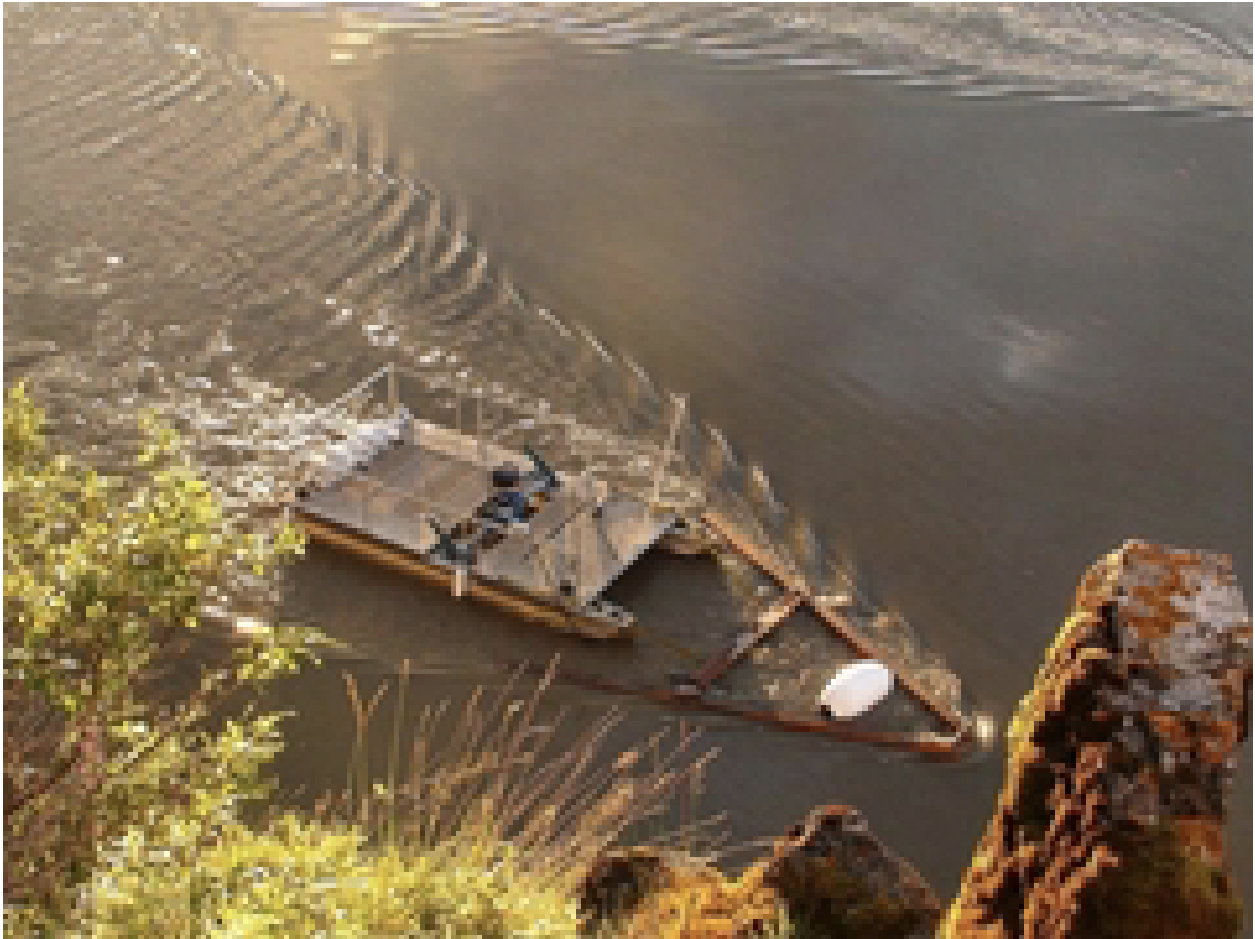
Figure 1.2: Debris boom on 5 kW Encurrent Turbine in Ruby, Alaska [18].
