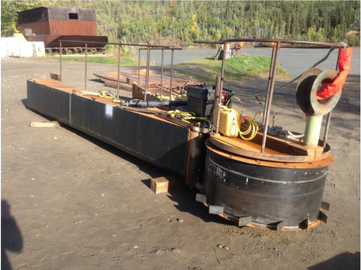
Figure 2.1: The RDDP debris sweep (front cylinder) and pontoons with plastic sheet covering to reduce contact friction between the RDDP and debris. [13].
