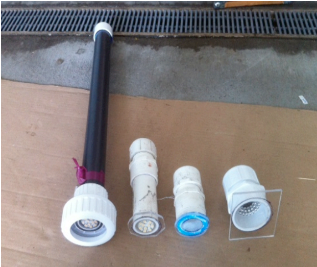
Figure 3: PVC light enclosures. Unit utilized most frequently is second from the left.
