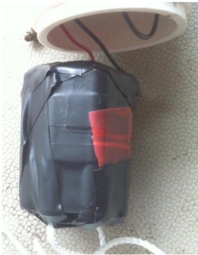
Figure 4: Power supply for most utilized light enclosure composed of 8AAA batteries soldered in series.
