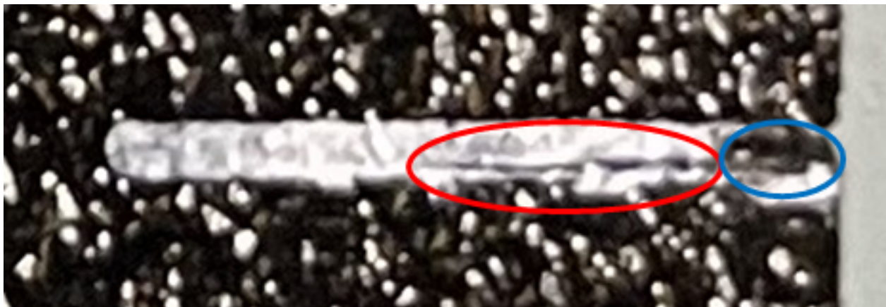
Figure 3.9: The extra damage created while cutting the notch. The blue circle is the notch cut by the razor saw, and the red circle is the extra barely visible damage in front of the crack tip.
