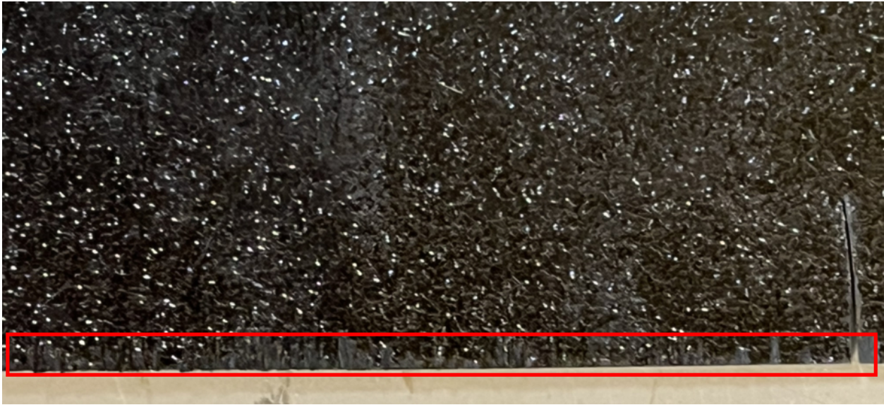
Figure 3.5: Zoomed photo of a SENT coupon. The fibers in the red box are stretched while being cut.
