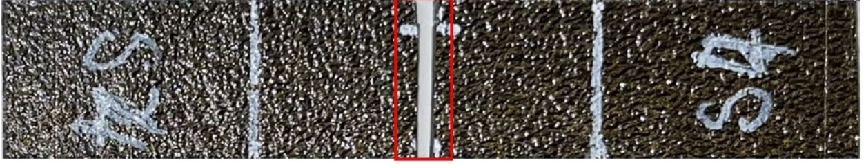
Figure 4.3: The photo of a tested small-sized SENT coupon, showing regular and crack in the middle of the coupon
