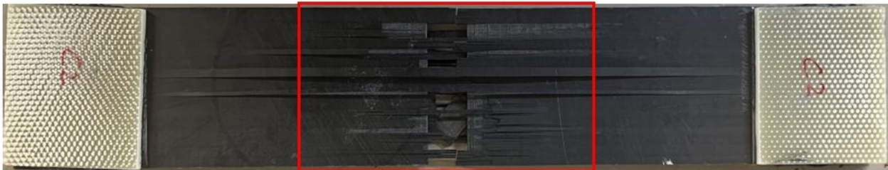
Figure 5.3: A DENT coupon after the test. The crack is irregular and fiber splitting significantly contributes to energy dissipation.
